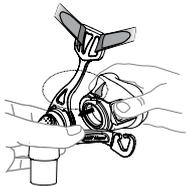
**1.** Align the two triangle and clip the cushion to the frame.
